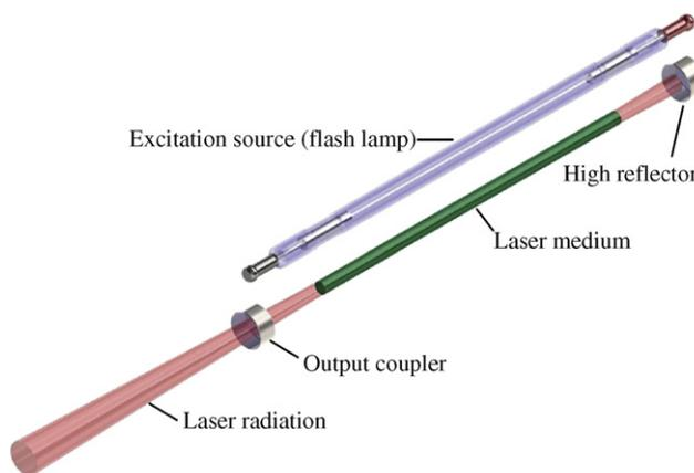
Fig. 2 – Optical resonator with excitation source (flash lamp). Green bar: laser medium; right end: high reflector; left end: output coupler; red beam: laser radiation. Courtesy of LISA Laser, Katlenburg, Germany.
