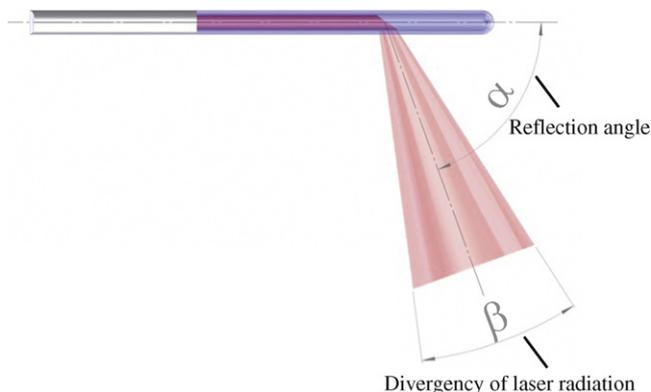
**Fig. 4 – Design of a side-firing fibre.  $\alpha$  = reflection angle,  $\beta$  = divergency of laser radiation.** Courtesy of LISA Laser, Katlenburg, Germany.
