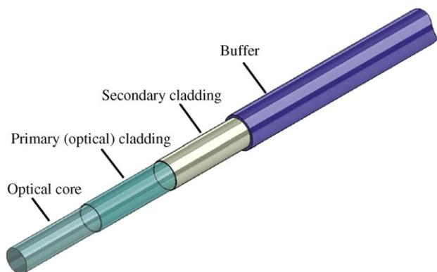
**Fig. 3 – Design of a front-firing fibre starting from the inner core: optical core (light blue), primary (optical) cladding (cyan), secondary cladding (silver), and buffer (indigo).** Courtesy of LISA Laser, Katlenburg, Germany.
